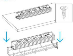
2. Fixate using one Philips screw M3x18 on each side
